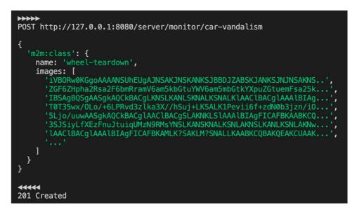
The Monitor AE creates a wheel teardown class inside the car-vandalism classifier including a set of images of cars with teardown wheels;
